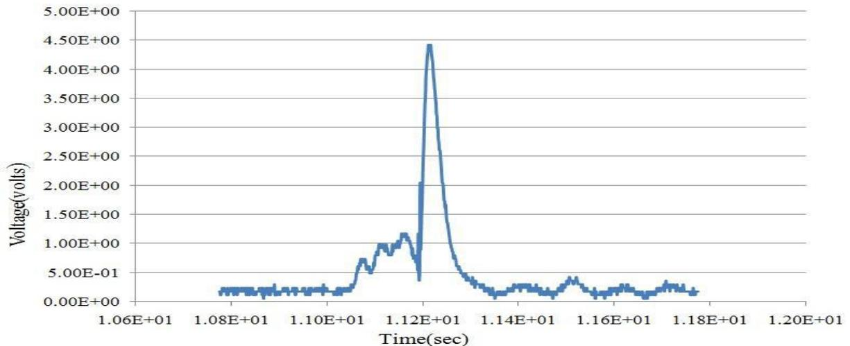
**Fig.5 Voltage vs time plot of PDE at 1 Hz with higher sampling rate**
