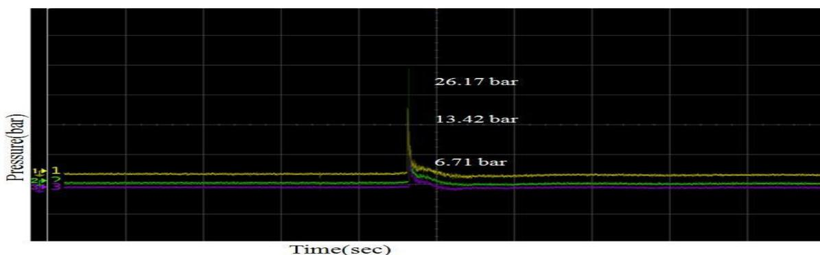
Fig.3. Pressure vs Time plot for PDE operated at 2 Hz
