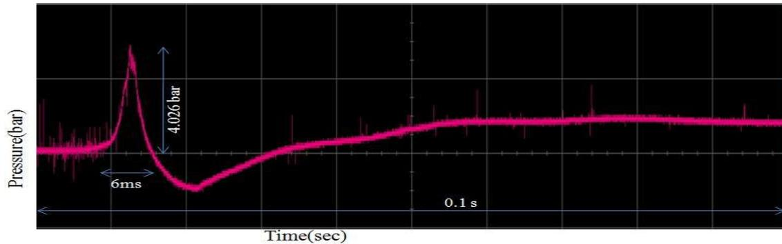
**Fig.6. Head end pressure captured for PDE at 1Hz with higher sampling rate**
