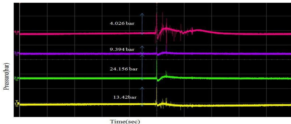
Fig.2. Pressure vs Time plot for PDE operated at 1 Hz
