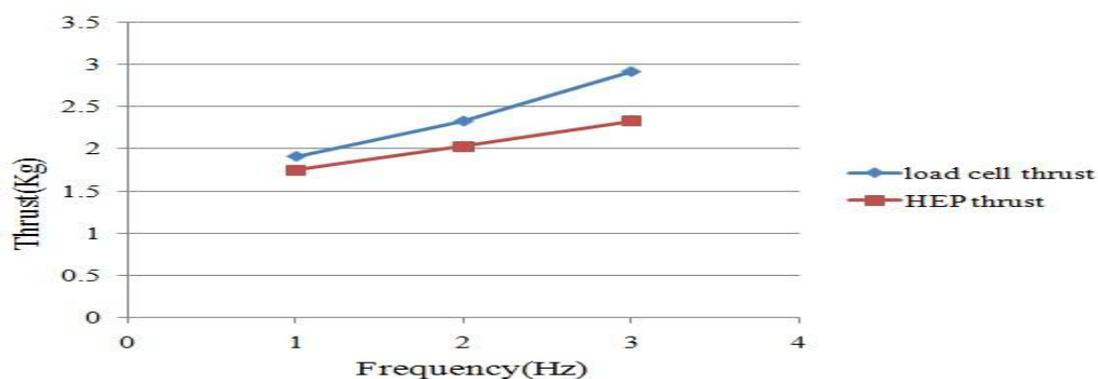
**Fig.7. Thrust variation with frequency**
