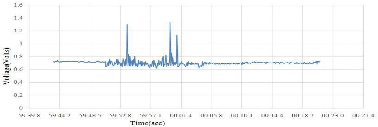
**Fig.4. Voltage vs time plot for PDE operation at 1Hz with lower sampling rate**
